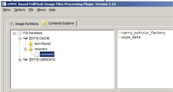
In order to perform factory reset, obviously such command must be written to any of supported locations so kernel can read it and execute on startup. To do this, we implemented universal method which search for MISC or PARA partition and uploads required commands to these partitions.
