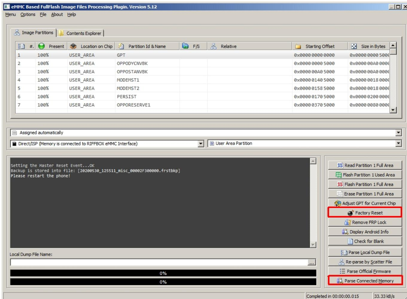
If factory reset is done over ISP connection, great care must be taken during shield removal and soldering. Approx 20% users can't do this properly and damage their (or their customers devices) usually by breaking resistors on CLK signal. In case that device doesn't turn on after assembling, make sure there is no physical damage to any parts in soldering area and that shield removal didn't damaged prints on board.
