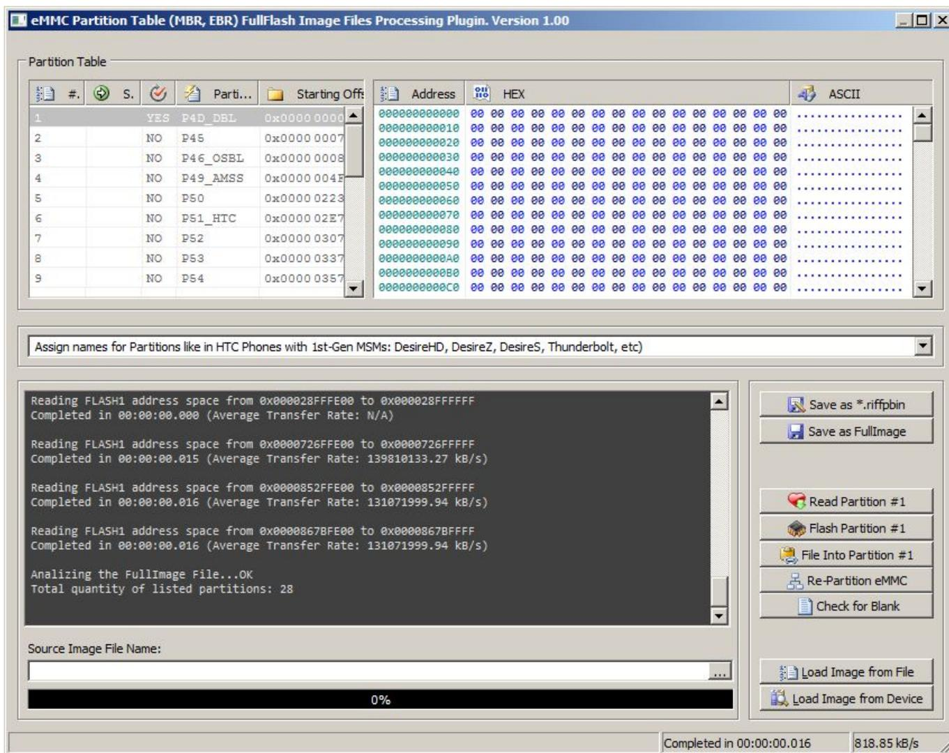
At this point an empty flash image will be created, filled with 00 00. Remember, this is just "placeholder" for actual flash content, and not a valid flash image.
