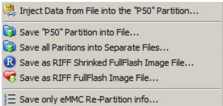
This will save "partition table", which can be used later for blank (erased or new) eMMC chips. **Take note, only file saved from working device is valid.**
