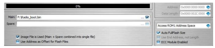
This option is used to automatically read flash chip size and apply values to address and length fields. When this option is checked, it disables address, data length fields, and "Use end address" option.
