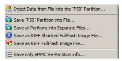
This will save "partition table", which can be used later for blank (erased or new) eMMC chips. **Take note, only file saved from working device is valid.**
