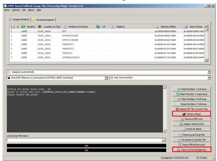
If factory reset is done over ISP connection, great care must be taken during shield removal and soldering. Aprox 20% users can't do this properly and damage their (or their customers devices) usually by breaking resistors on CLK signal. In case that device doesn't turn on after assembling, make sure there is no physical damage to any parts in soldering area and that shield removal didn't damaged prints on board.
